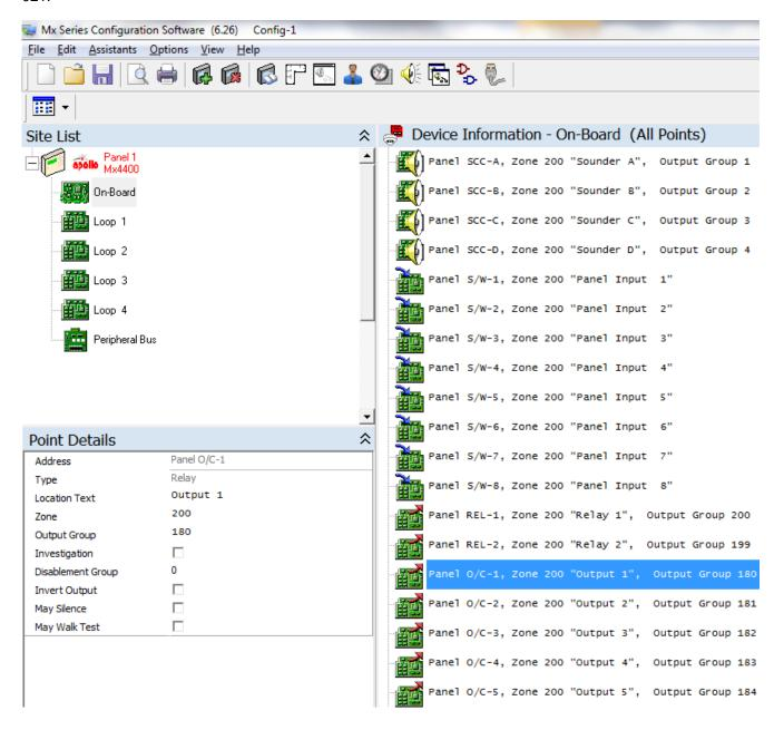
The properties that can be assigned to each relay output are depicted in the boxes on the "Point Details" section. By ticking the appropriate box, the relay will take on those assigned properties.
