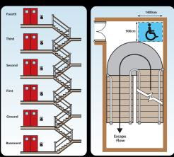
Examples of a Type B outstation installed in the protected stairway providing egress from each storey
